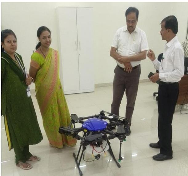
On the left side snap we see Dr. S Hegde sir from CUK showing the Dorne used for fertilize purpose at farm, using this drone which hold's 5 liter liquid capacity to fill the pesticides & spray the same over the farms as an innovation towards automation
